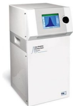
Fig. 2. a) Picture of the TSI EEPS model analyzer; b) MSS by AVL sensor [AVL 2017, TSI 2016]
