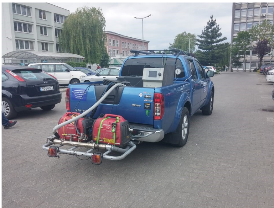
Fig. 1. The vehicle used in testing with PEMS equipment
