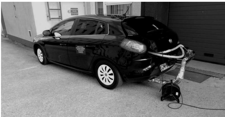
Fig. 1. The vehicle used in testing with SEMTECH equipment
