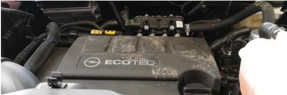
Fig. 2. The injectors placement in Opel Mokka
