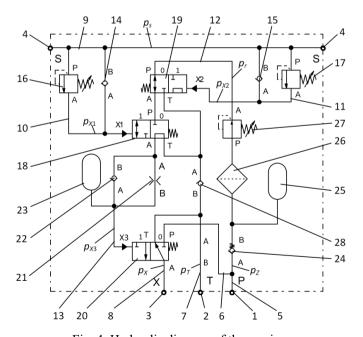
Fig. 4. Hydraulic diagram of the receiver
