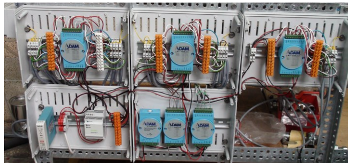
Fig. 15. Adam series 4117 and 4118 modules, USB-RS232 converter and the adapters
