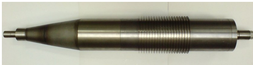
Fig. 7. The inner part of a single-sided seal: a) overview, b) image of the inner part with the discs and distance sleeves
