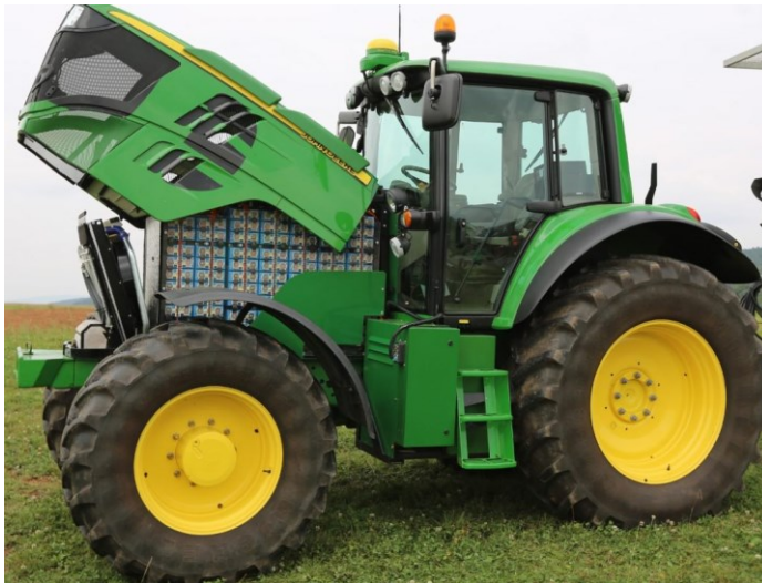
Fig. 3. Example of an electric drive system in an agricultural tractor [John Deere 2016]
