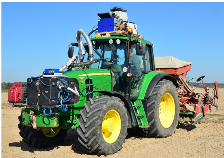
Fig. 5. Example of using PEMS during farm tractor test
