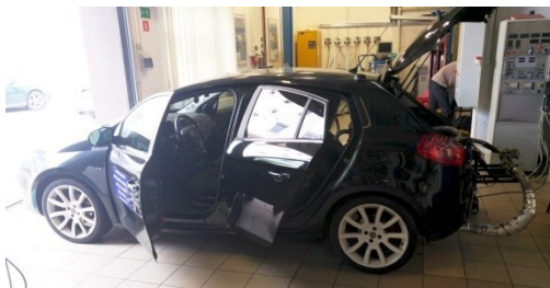
Fig. 1. Vehicles used in testing with PEMS equipment: a) Fiat Bravo, b) Saab 9-3
