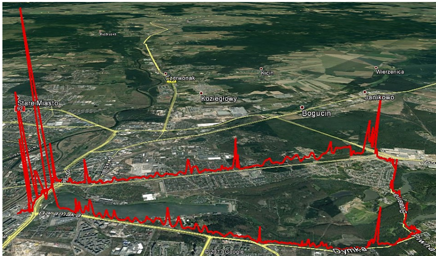
Fig. 8. Results of the CO emissions during Saab 9-3 drive
