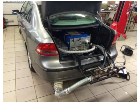
Fig. 1. Vehicles used in testing with PEMS equipment: a) Fiat Bravo, b) Saab 9-3
