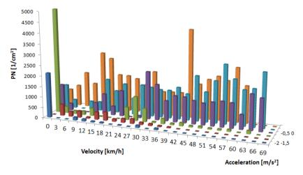
Fig. 14. Emission of PN in the range of vehicle speed and acceleration during economic drive
