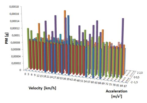
Fig. 13. Emission of PM in the range of vehicle speed and acceleration during economic drive
