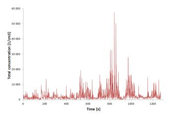
Fig. 6. Total concentration of PM during dynamic drive
