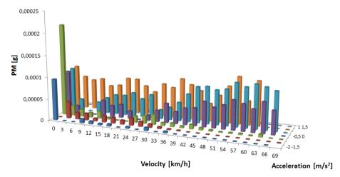
Fig. 12. Emission of PM in the range of vehicle speed and acceleration during dynamic drive
