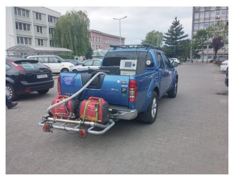
Fig. 1. The vehicle used in testing with PEMS equipment
