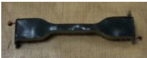
Fig. 3. The extruded material produced with a die (dumbbell specimen)
