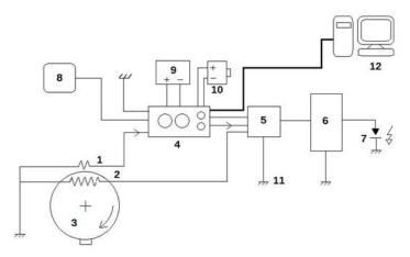
Fig. 1. Diagram of the digital ignition system utilized: 1 – pulse generator, 2 – generator coil, 3 – generator with a marker, 4 – microcontroller, 5 – CDI module, 6 – ignition coil, 7 – spark plug, 8 – throttle, 9 – battery, 10 – starter, 11 – ground, 12 – PC
