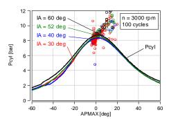
Fig. 4. The impact of changes in the ignition angle of advance on the characteristics of combustion pressure and dispersion of  $P_{max}$  in the cylinder: a) at n = 1900 rpm, b) at n = 3000 rpm
