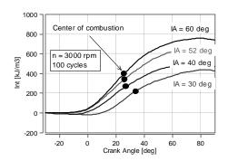
Fig. 6. Changes in the heat generation and determination of the centre of combustion: a) at n = 1900 rpm, b) at n = 3000 rpm for variable ignition angle of advance
