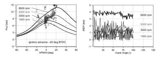
Fig. 7. Characteristics of engine speed at a constant ignition angle of advance: a) changes of the cylinder pressure, b) changes of IMEP in successive cycles of engine operation
