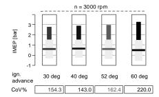
Fig. 5. Dispersion and values of the coefficient of variation of the mean indicated pressure: a) at n = 1900 rpm, b) at n = 3000 rpm
