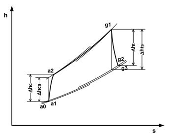
Fig. 2. Gas turbine 'cycle', enthalpy-entropy diagram
