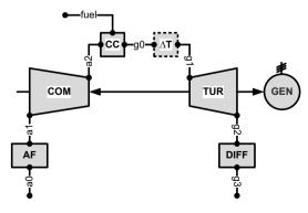
Fig. 1. Model of a gas turbine unit
