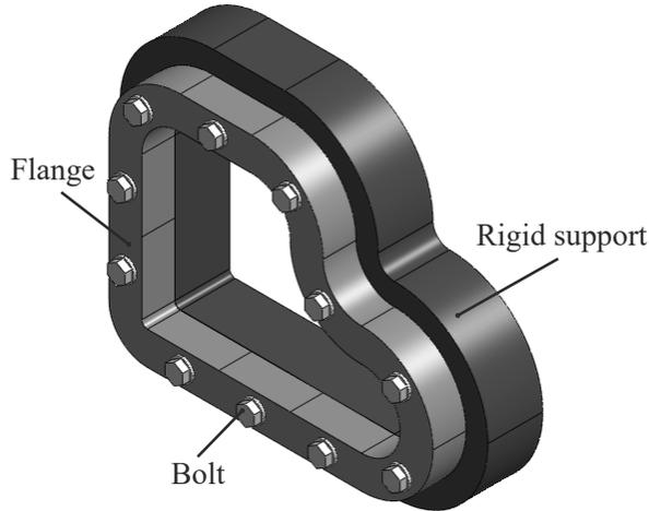
Fig. 1. Example of a bolted flange connection
