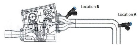
Fig. 1. The investigated injector positions; A - 60 cm away from intake valve, B - 10 cm from intake valve
