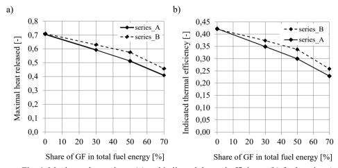
Fig. 4. Maximum heat release (a) and indicated thermal efficiency (b) for location A (full-line) and for location B (dashed-line)
