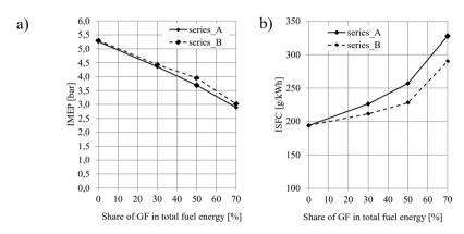
Fig. 3. IMEP (a) and ISFC(b) in series A (full-line) and series B (dashed-line)
