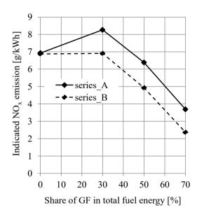
Fig. 5. The comparison of NO<sub>x</sub> emissions in location A (full-line) and location B (dashed-line)
