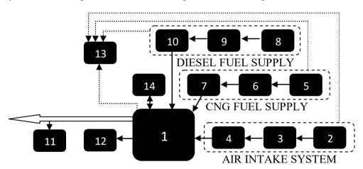
Fig. 2. Engine test stand with measurement equipment; 1 – AVL 5804 engine, 2 – air filter, 3 – air mass flow meter, 4 – full-variable supercharging system, 5 – CNG vessel, 6 – CNG mass flow meter, 7 – injector, 8 – diesel tank, 9 – gravimetric diesel fuel mass flow meter, 10 – common-rail diesel injection system, 11 – Horiba Mexa exhaust gas analyser, 12 – engine indicating system, 13 – temperatures and pressures monitoring system, 14 – engine control system
