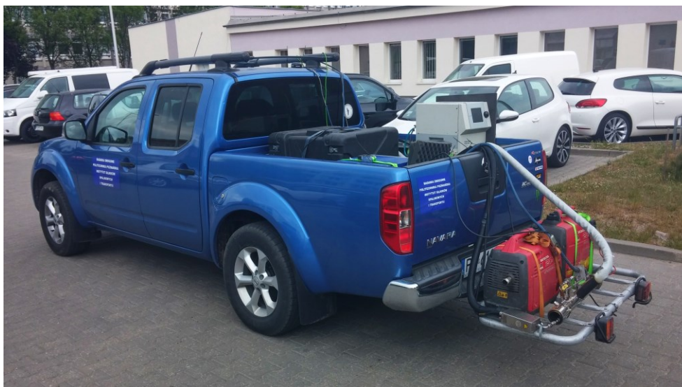
Fig. 1. The vehicle used in testing with PEMS equipment
