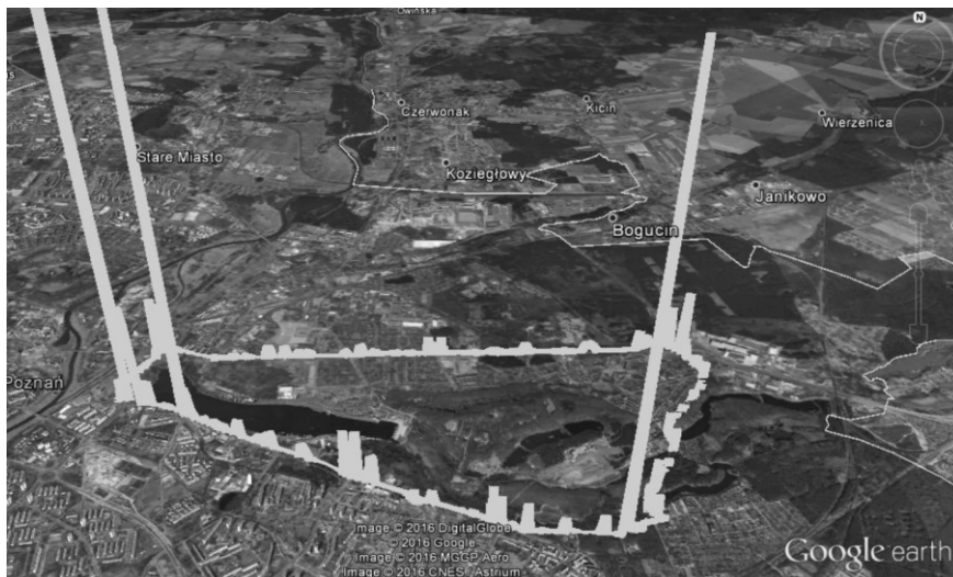
Fig. 5. Results of the CO emissions during dynamic drive
