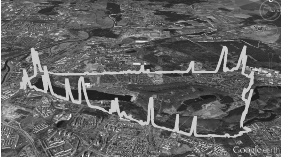
Fig. 6. Results of the \text{NO}_x emissions during dynamic drive
