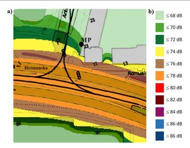
Fig. 4. a) The first acoustic map representing the traffic noise levels around the measuring point MP at the height of 8 m over the ground, b) Range of colors assigned along with the equivalent sound pressure A levels  $L_{Aeq}$
