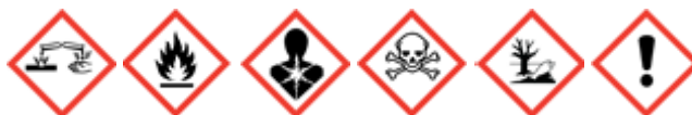
Fig. 3 Pictograms used in the European Union (GHS) on the packaging which contains hydrazine [European Chemicals... 2017]
