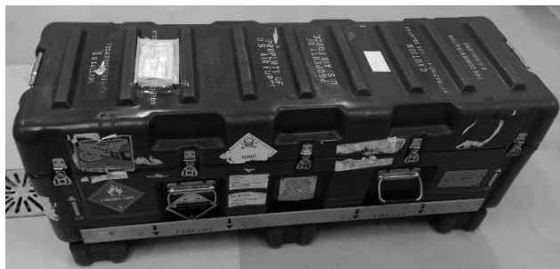
Fig. 2. Transport container for hydrazine gas cylinder
