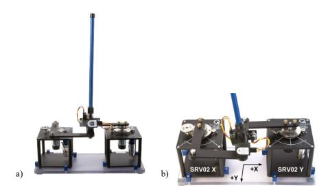
Fig. 1: The test stand [Quanser 2012]
