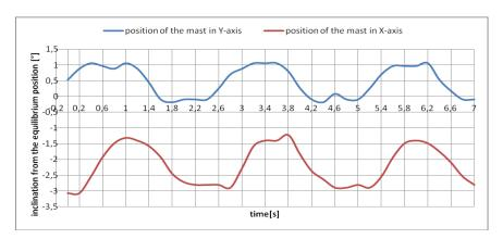
Graph 2. Position of the mast of the inverted pendulum during the stationary test [Judt 2015]
