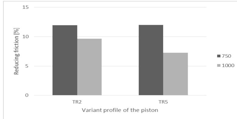
Fig. 4. Percentage reduction of total losses piston ring package with a modified geometry as a function of engine speed
